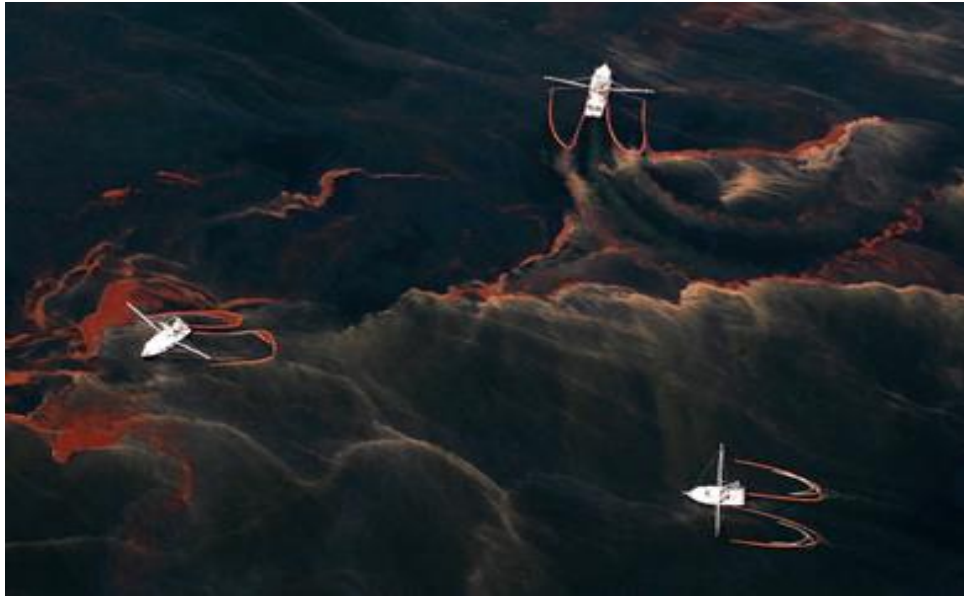
Figure 26. Fishing vessels with booms and sweeps to collect surface oil (Macondo Oil Spill)
