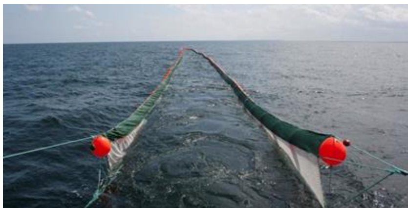
Figure 24. NetBoom used for the collection of oiled Binders
