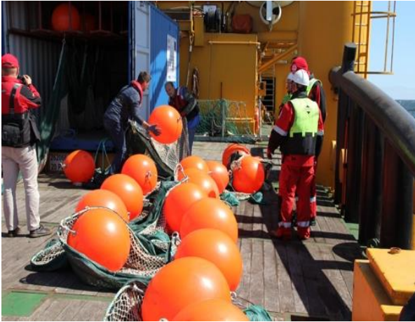
Figure 10: The boom is discharged from container
