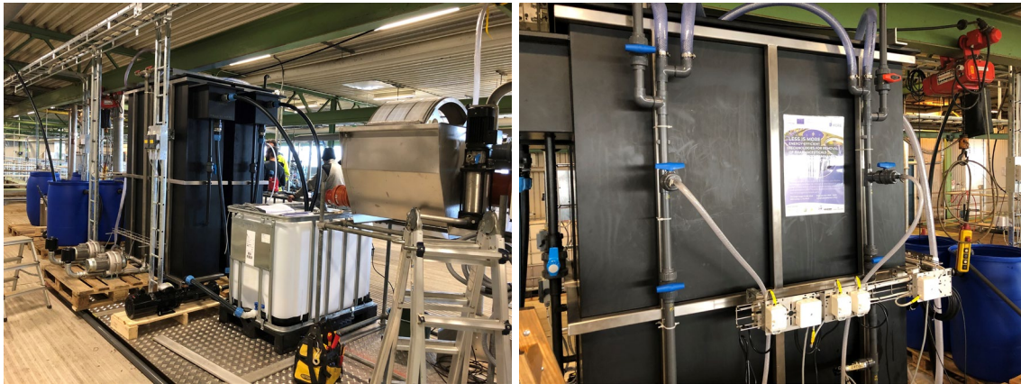
Figure 4. The pilot plant in Svedala, Sweden. The left picture shows the drumfilter, the equalization tank, the membrane unit (black) and the GAC-filters with equalization tanks in blue at the far end. The right picture illustrates the membrane unit.
