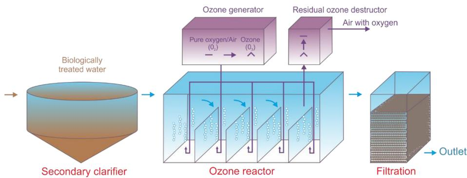
Figure 2. Schematic overview of the ozone unit suggested location in the conventional wastewater treatment technology (modified from<sup>13</sup>)
