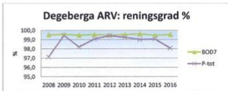
Figure 2. Treatment efficiency of BOD<sub>7</sub> and P<sub>tot</sub> at Degeberga WWTP 2008-2016. Graph from Degeberga WWTP Environmental Report 2016.
