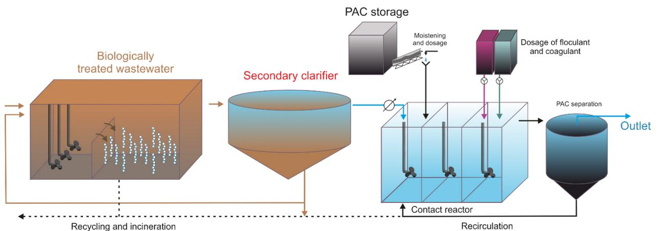
Figure 3. Schematic overview of the PAC unit suggested location in the conventional wastewater treatment technology (modified from<sup>14</sup>)
