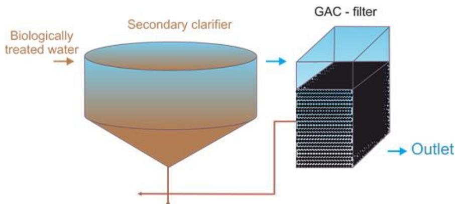
Figure 4. Schematic overview of the GAC unit suggested location in the conventional wastewater treatment technology (modified from<sup>15</sup>)
