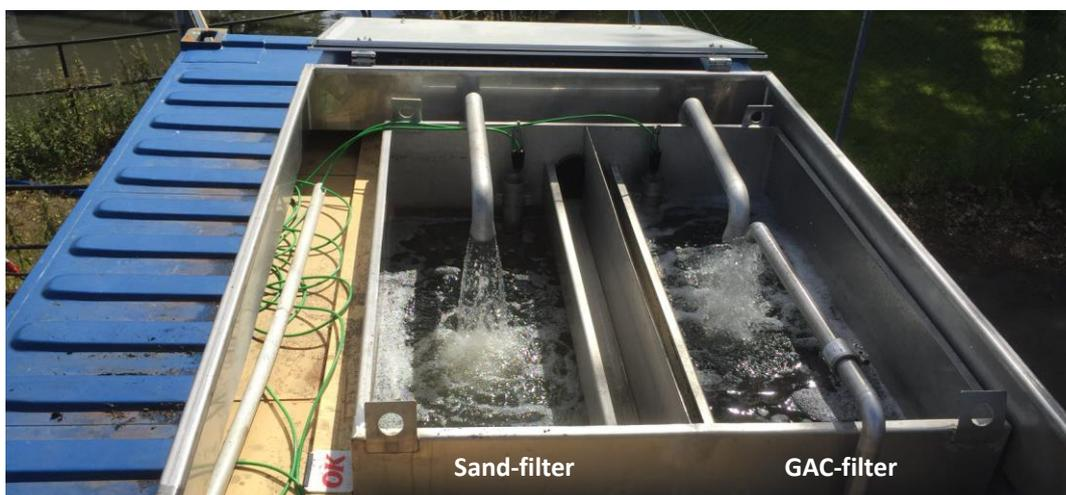
Figure 5. Pilot-scale plant in operation at a flow of 2m<sup>3</sup>/h. To the left 1 m<sup>3</sup> of sand as a pre-filter step followed by 1 m<sup>3</sup> GAC to the right. Photo: Erland Björklund.
