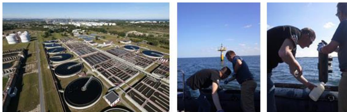
Figure 3.7 From left Gdansk-Wschod WWTP, with sampling of the discharge point – marine outfall into Gdansk Bay (Nansen bottle was used for bottom and surface water collection)
